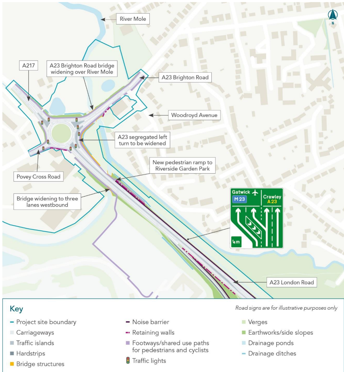
Figure 2.5 : Proposed Longbridge Roundabout improvements
