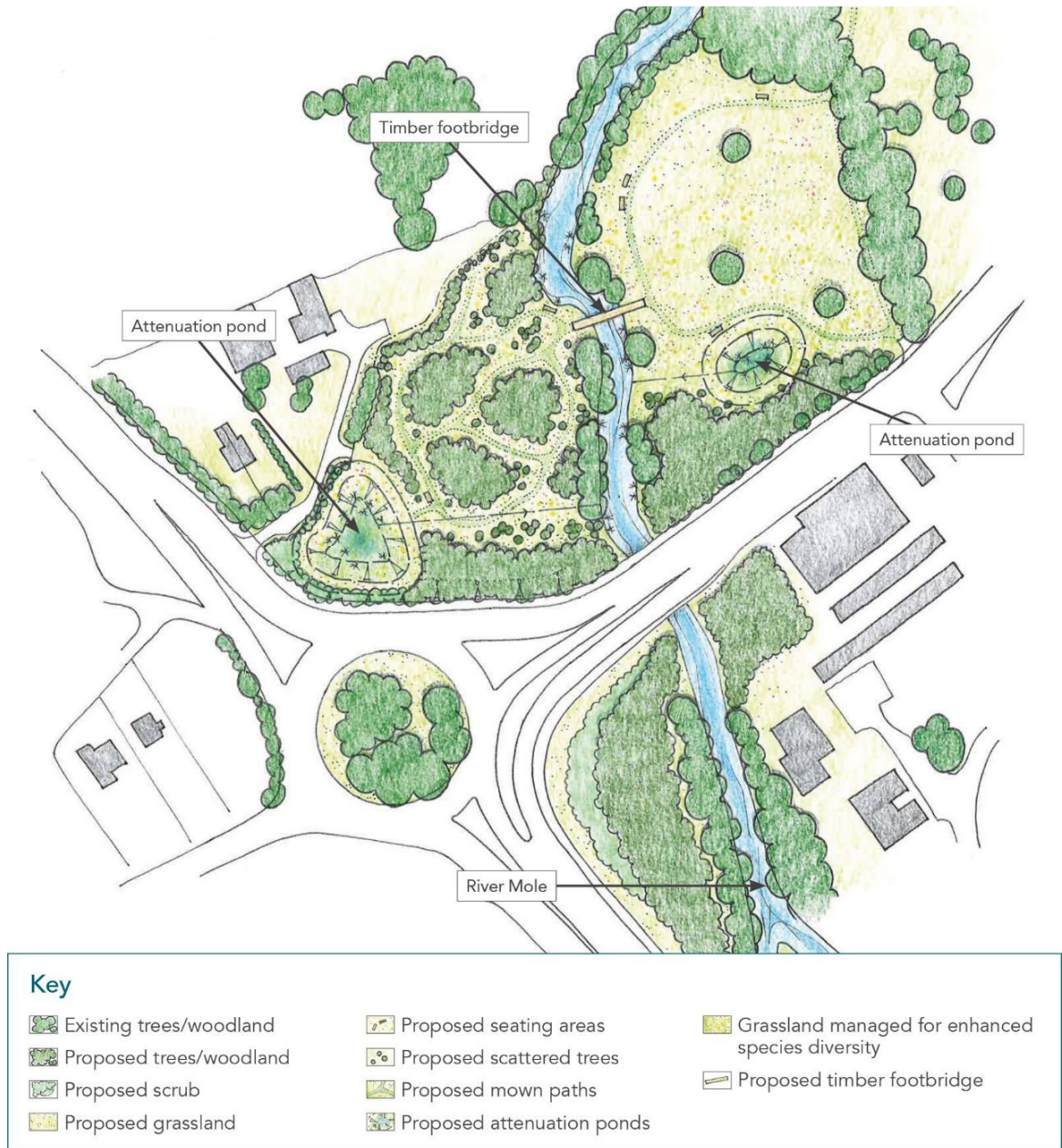
Figure 3.6 : Integrated concept mitigation designs for Church Meadows
